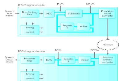
11. Diagram of differential pulse code modulation encoder and decoder. [D] [Nov/Dec-2017]
